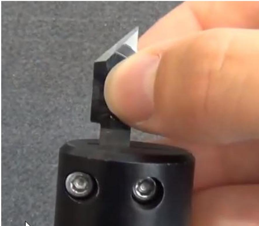
5. Press the button (1) and insert the tool back into the module. Turn the knob until the pin falls in the slot. (2)
