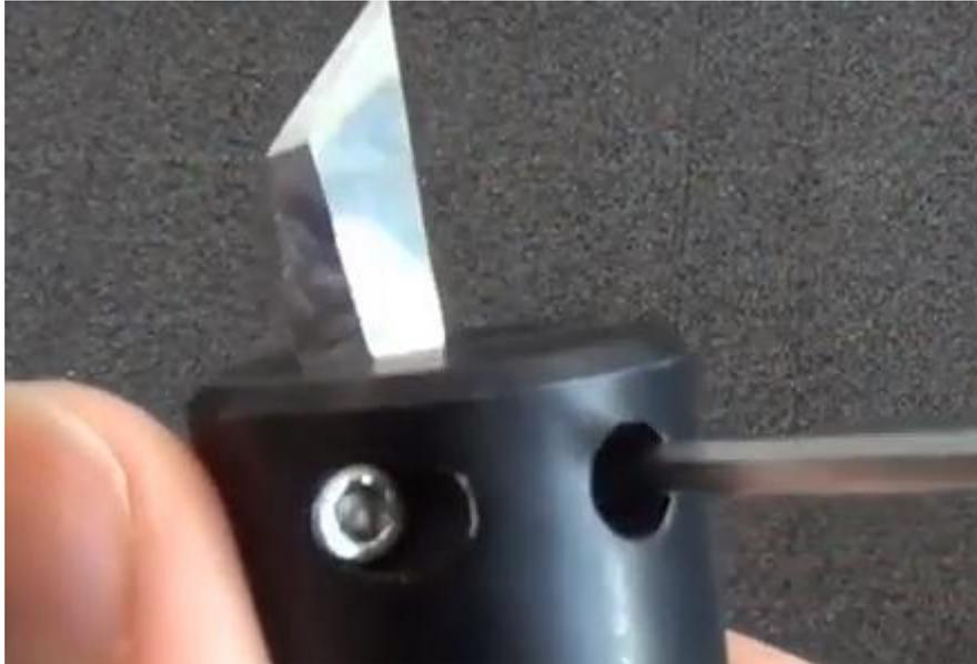
4. Carefully remove the knife. Position the point in the middle of the holder and tighten the two screws.
