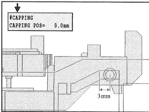
2. Make adjustment so that the cap slider is located at 3 mm to the right from the uppermost point it has reached on the cap base.
