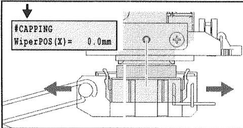
5. Make adjustment so that each center of the wiper and the head coincides.
