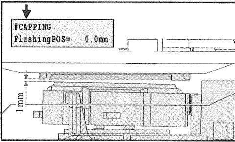
4. Make adjustment so that the clearance between the head and left end of the cap is set at 1 mm.
