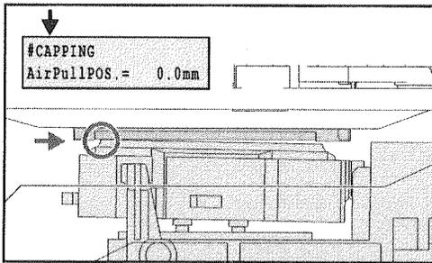
3. Make adjustment so that the head is located exactly at the point where the head is in contact with rubber portion (left end) of the cap head.
