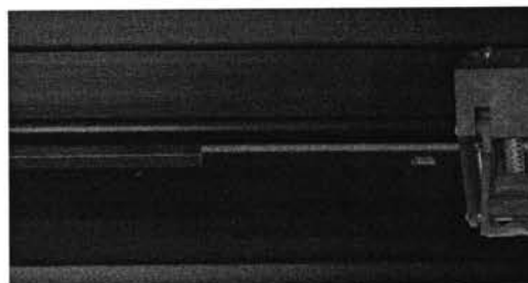
FIGURE 6 PLACE MADE FOR EXTRA PINCH ROLLER
