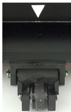
Defective pinch roller Out of center
