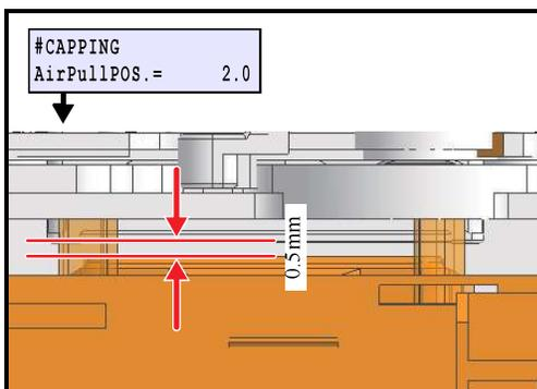
3. Make adjustment so that the clearance between the head and uppermost point of the cap is set at 0.5 mm.
