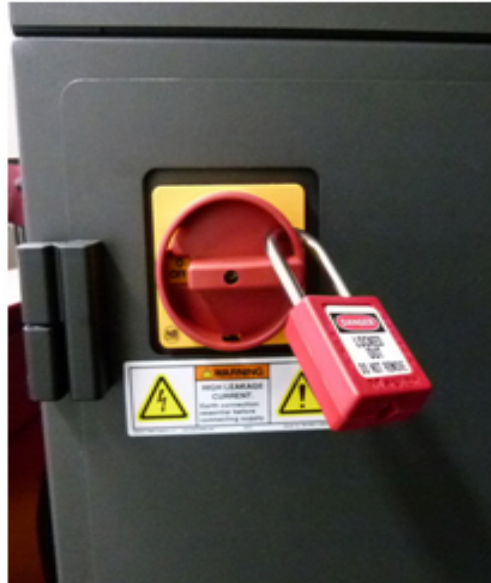
Figure 2: Main disconnect switch-lockout/tagout in the OFF position (shown here on a TX3250r model printer)
