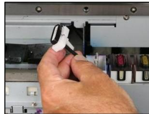
14. Carefully feed the new **Cap Top** into the hole inside the **Cap Station Assembly** and direct the **Cap Top Tube** down so it can be pulled
