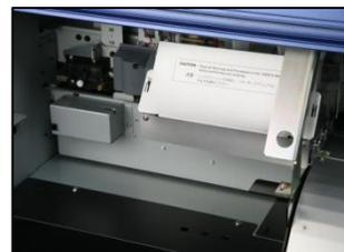
6. The head carriage will move down to the far end of the machine on its own at this point and will be out of the way.
