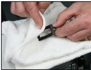
9. Clean the **Cap Frame Cover** with a paper towel or cleaning solution if needed.
