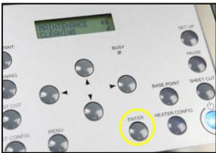
21. Press **ENTER** to end the **MAINTENANCE CLEANING** procedure.
