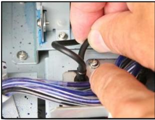
19. Connect the **Ink Tube** from the new **Cap Top** to the **Y Adaptor**.
