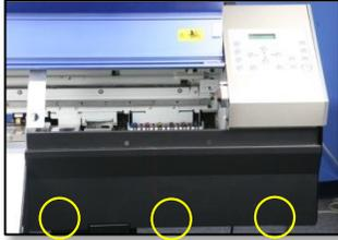
7. Remove the **Pump Cover** below the **Cap Station** (3 screws) and set aside.
