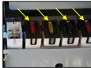
13. Note carefully the orientation of the **Cap Top**, the hole in **Cap Top** positioned to rear of assembly.
