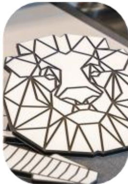
Engraving with folding bit
