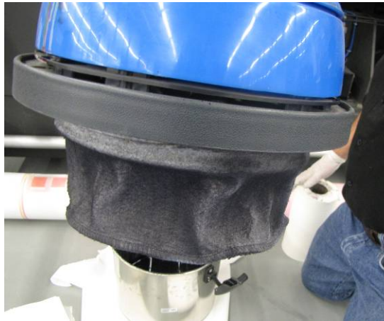
Remove Top, Remove Lower Filter and Seal
