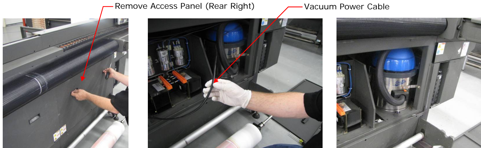
Figure 3: Accessing The Vacuum Canister
