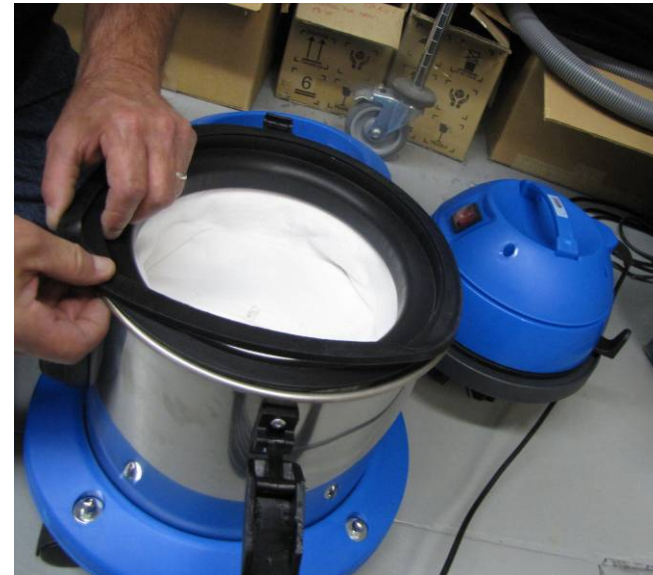
Figure 13: White Filter and Rubber Seal
