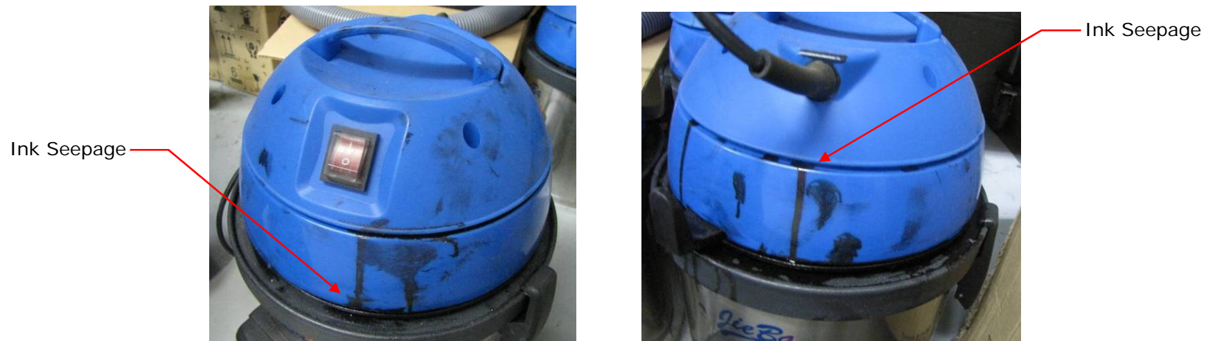
Figure 6: Vacuum Canisters Requiring Replacement
