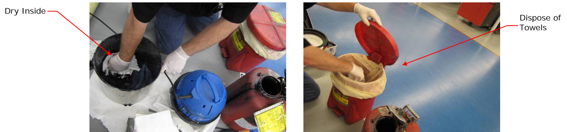
Figure 10: Emptying the Vacuum Canister
