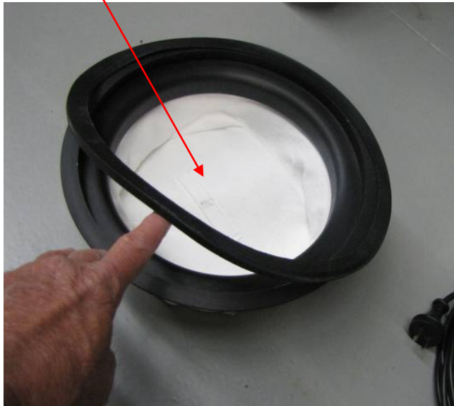
Figure 13: White Filter and Rubber Seal
