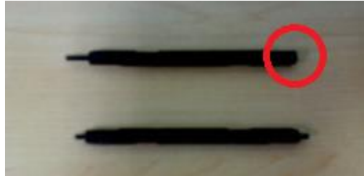
Broken Pinch Wheel
