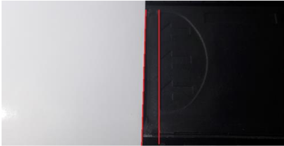
Media not moving parallel through print zone
