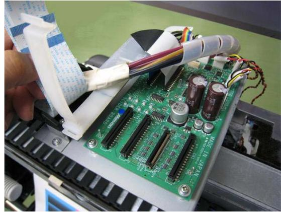
(4) Apply the double-stick tape to the following position in the order of Photo A to C and fix 4 FFC as the Photo D.
