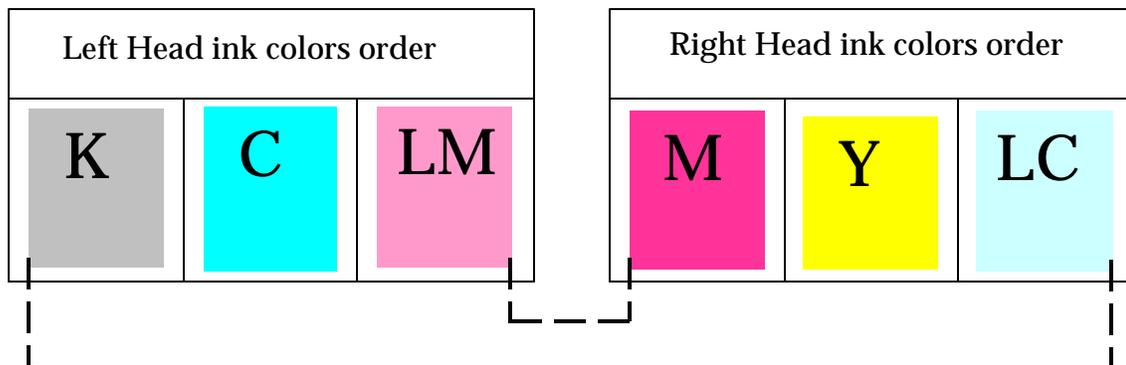
To perform the mechanical alignment of the left head to the right head.
