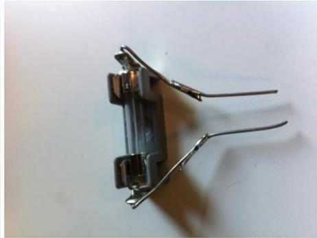
Cut off resistor and throw it away. Use other wires from the other resistors to make fuse holder longer.
