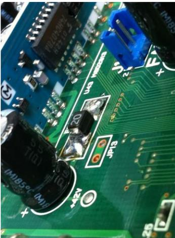
Once located use solder gun to build up the solder on both sides of the fuse so the wires will have something to solder to. Don't worry about removing old fuse as it is bad and not necessary. See picture and see mound of solder.
