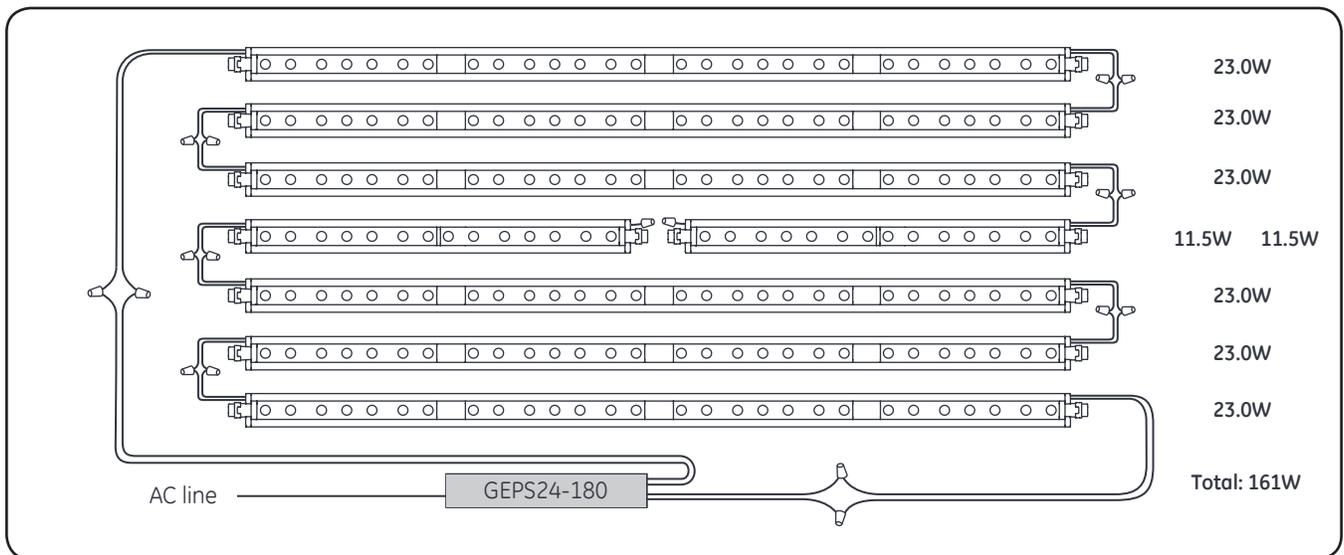
**5** Connect Line Fit Lights using twist-on wire connectors or in-line (IDC) connectors. Join white wires together and red striped wires together. Cap all exposed wires with appropriate end caps or apply electric grade (non-corrosive) silicone for additional weather protection.
