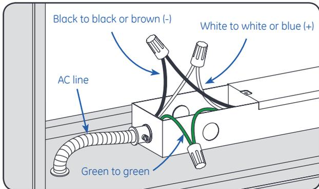
**3** Wire AC line to LED driver(s) in accordance with the applicable local, state, and country electrical codes. Connect black to black or brown, white to white or blue, and green to green using 18 AWG (0.82mm<sup>2</sup>) wire connectors.
