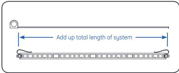
**1** Add up total footage of the system to determine the appropriate number of 24VDC Class 2 Tetra® LED drivers to use based on the **Power Supply Loading** chart on last page.
