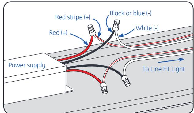
**4** Connect the red stripe wire (+) of the LED system to the red wire (+) of the power supply. Connect the white wire (-) of the LED system to the black or blue wire (-) of the power supply.
