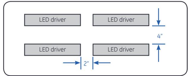
**2** If installing multiple LED drivers, keep them at least 2" (50.8mm) apart end to end and 4" (101.6mm) apart along the sides.
