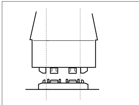
Make sure the HEADs are capped correctly.
