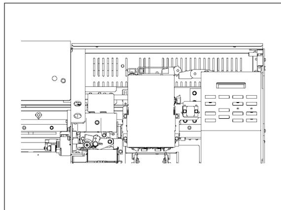
**9** Adjust the position of CAPPING UNIT by moving it left and right by hand so that the caps come straight below the each head.
