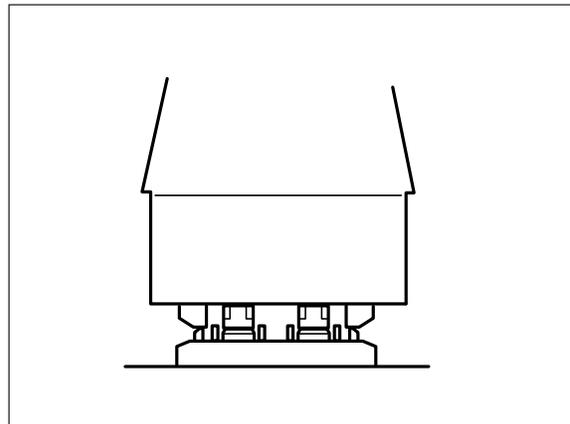
**10** Fix the four screws for fixing the CAPPING UNIT at that position.
