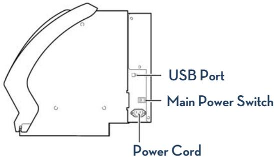
2. Connect the USB cable to the printer and the PC and then turn ON the printer's main and sub power. Windows will detect that a new device has been connected to the computer and will try to locate the driver. No user action is required if you are running Windows 7. If you are running Windows Vista and are prompted to locate the driver, select to not install the driver.
