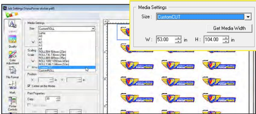
C. Once the width has been recorded, select the [Size] drop down and select [Custom Cut]. Notice that the width of the setup has changed back to the default width (max of the printer) and the height changed to 104”.
