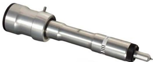
The Fiber Tip Tool option provides drawing capabilities on materials such as clear vinyl, which normally cannot be marked with ballpoint or liquid ink pens. It uses a standard Staedtler Lumocolor fiber tip drawing pens, which comes in different line weights. Line thickness will be less consistent than with the liquid ink cartridges due to the properties of the relatively soft fiber tip. The Fiber Tip Tool comes with 8 multi-colored pens included.
