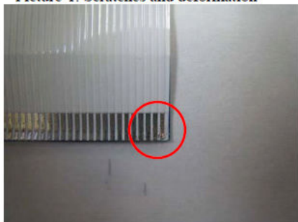
Picture-1. Scratches and deformation
