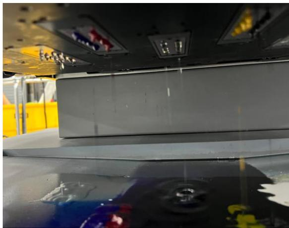
Using a folded lint free cloth start at the back of each head and wipe forward. Make sure to use a clean section of the cloth for each head so you do not cross contaminate inks.
