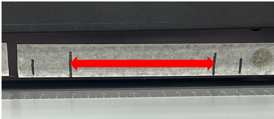
Look for missing or deflected nozzles. Purge again if needed or you can print the file “CMYK\_WH\_CL PURGE PRINT.CDL” and it will print a solid block pattern of each head. See examples of a bad and good nozzle pattern below.
