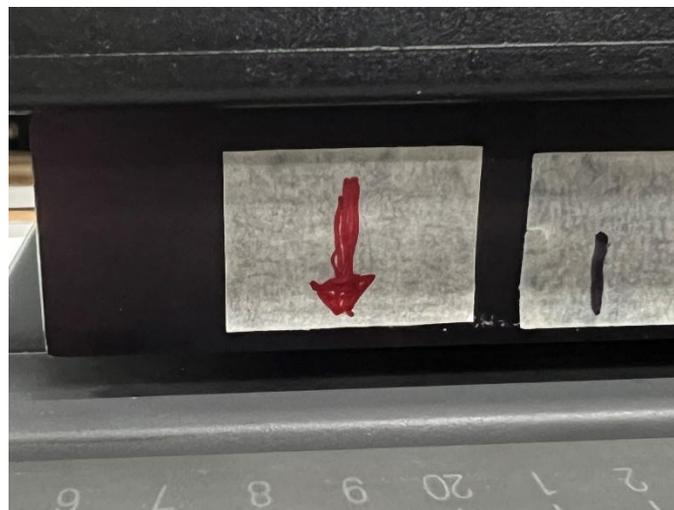
Make sure to position the carriage so that the circular pad is directly over the area you need to measure. You do this by holding down the CTRL button and any one of the arrow keys depending on which direction you need to move it. Make sure it will contact the substrate completely and not miss it in any way. Failure to do this may result in the carriage being put out of alignment. Double check its location before moving to next step.
