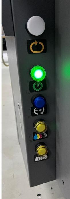
Then push the blue button below it. The blue button is also pushed after an error such as resetting the printer after the red stop button on the carriage has been pushed due to a head strike or other stoppage and manually moved back to its home position. Make sure status light at top of carriage turns to solid amber.
