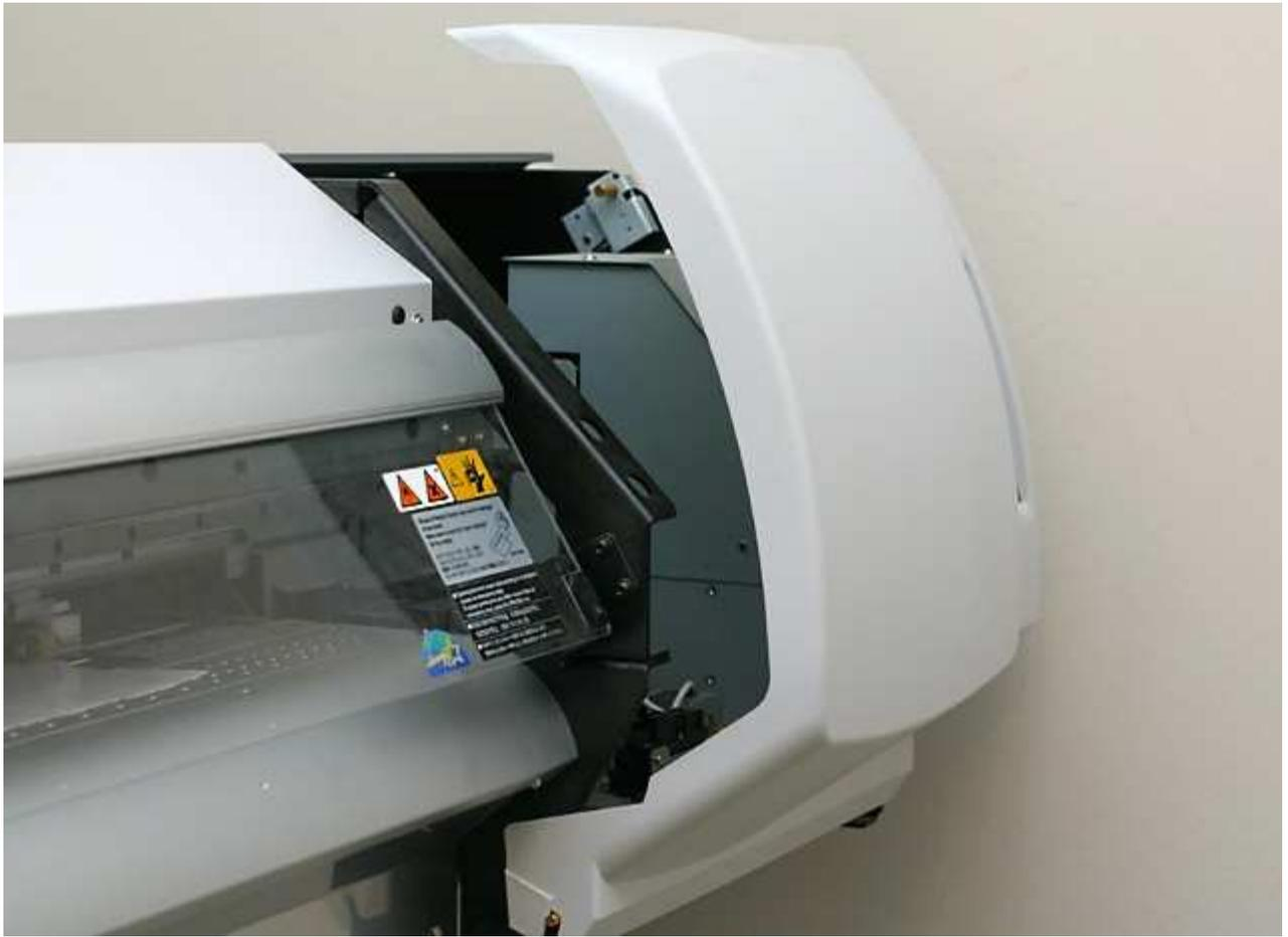
Looking into the main carriage of the unit you should see your exposed capping station.
