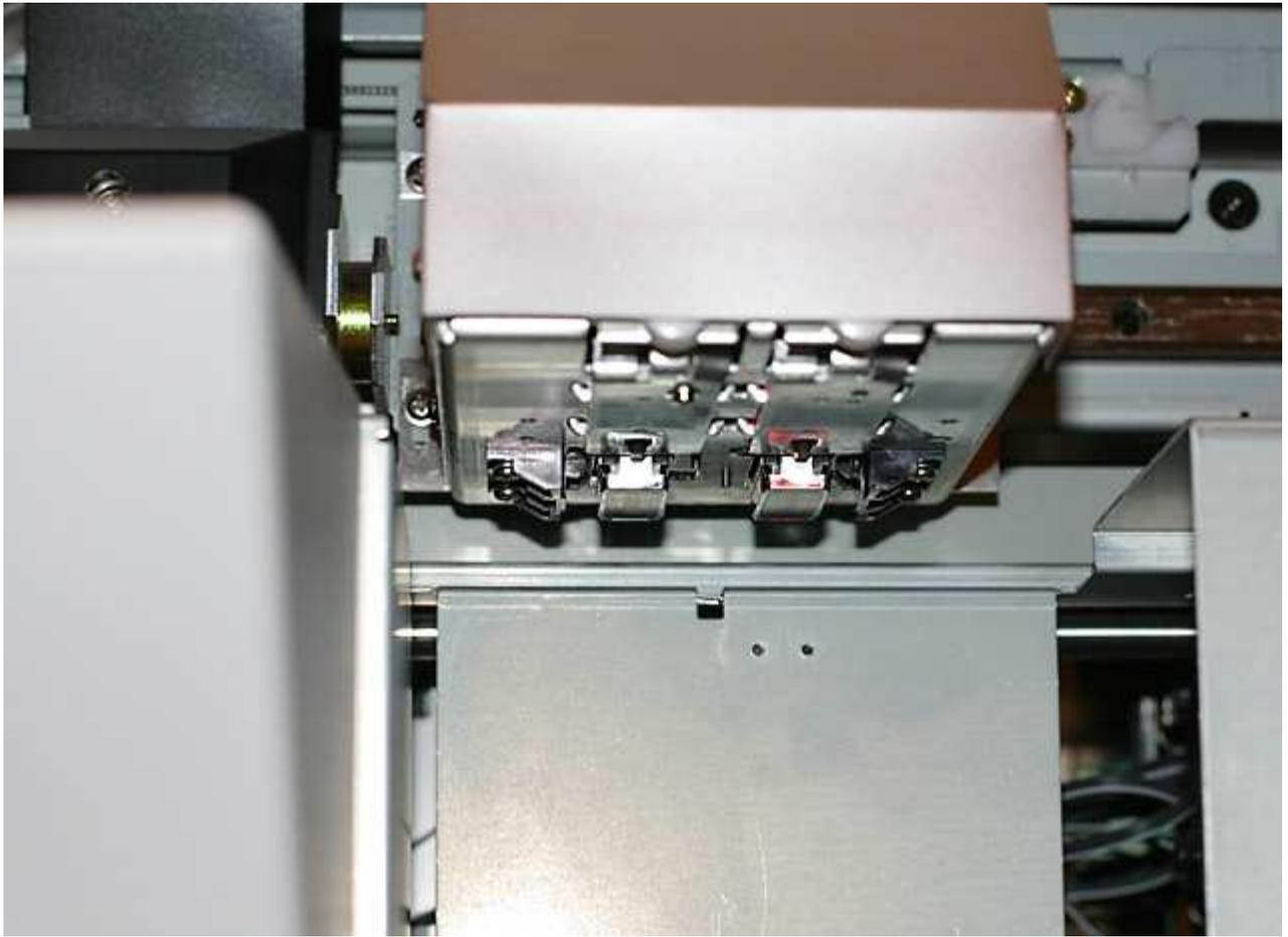
Take one of your solvent cleaning swabs and place a few drops of cleaning solution on the tip. Wipe around the edge of the heads being careful not to touch the bottom of the heads. **Touching the of the heads can push debris into the [nozzles](#) and clog them.** Using a small flashlight inspect for any fuzz or other debris hanging off the edge and remove it.
