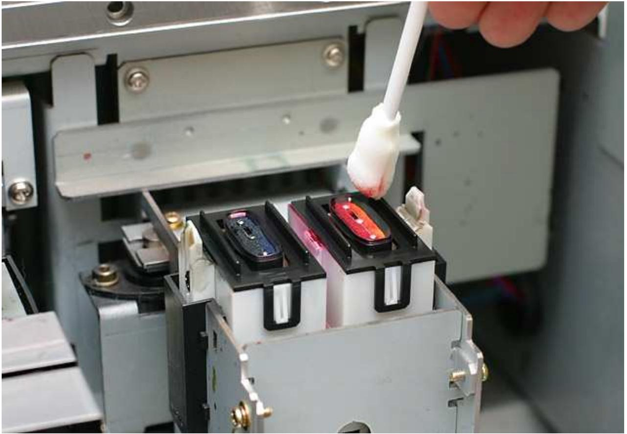
Next take your bottle of cleaning solution and fill the capping station to the top with cleaning fluid. Do not overflow the capping station; just fill it to the top. This will help clean the bottom of your pump once the carriage is parked again. Also as the cleaning solution is pumped out of the capping station, it will help clean the internals of your pump.
