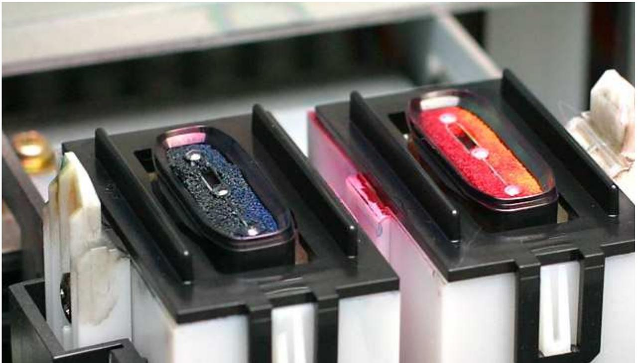
With a fresh cleaning swab (again with a few drops of cleaning solution) clean around the outer the capping station. This is where the head rests when it is parked and needs to remain clean. **to clean the around capping station can lead to problems down the road.**
