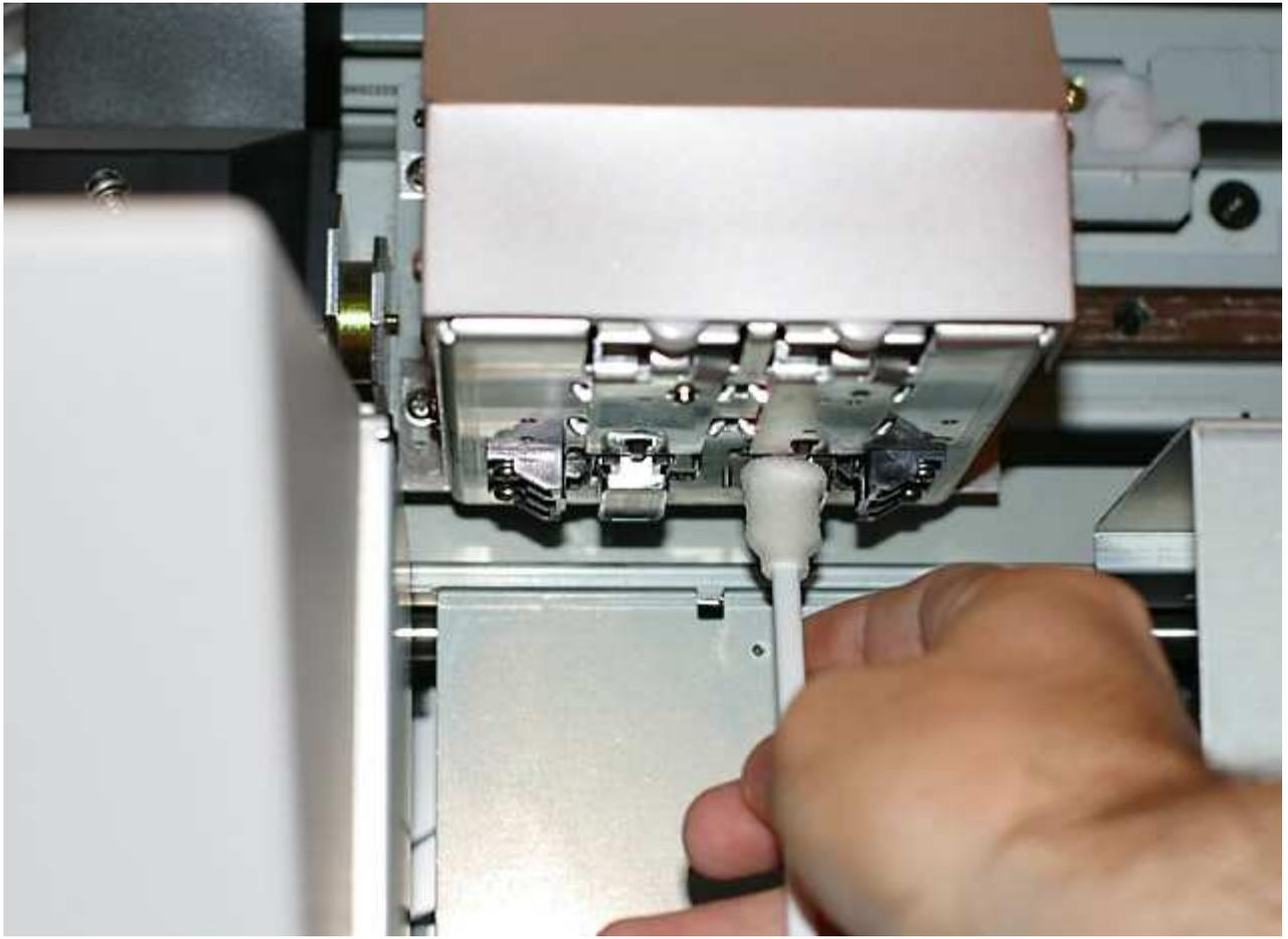
Once you have finished cleaning your heads open the front cover of your machine by removing thumb screws at the top. **Completely remove the cover and set it aside, the photo only shows it partially open.**
