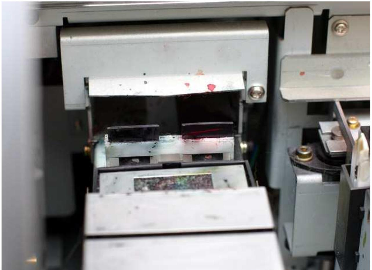
Using a cleaning swab with a few drops of cleaning solution clean only the front side of the wiper. Do not clean the felt back side of the wiper. (Note: if you are using full rubber wipers you should clean both front and back of the wipers). The wipers are what clean the bottom of your heads and need to remain clean. You may notice some fuzz build up on the wipers which can be removed with tweezers. If your wipers are sagging, cupping or do not have a straight edge they should be replaced.
