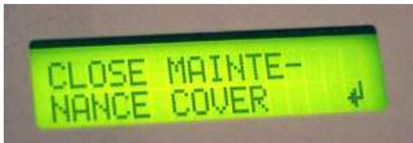
Place the maintenance cover back on and press **[ENTER]**. The machine will now power off and have completed your cleaning.
