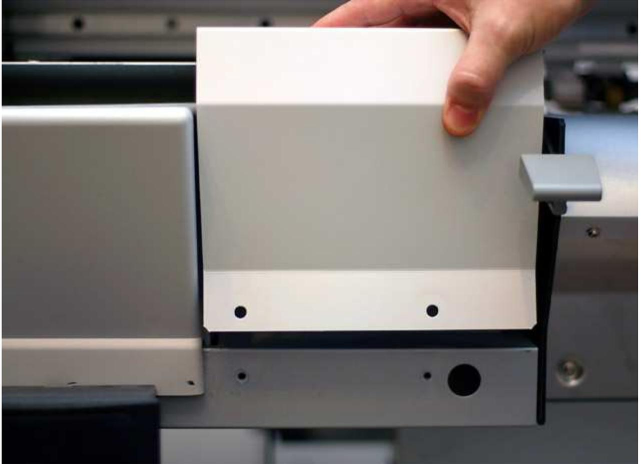
Press **[ENTER]** and your [print head](#) will move all the way to the left hand side of the machine you will be able to see the heads where the maintenance cover was.
