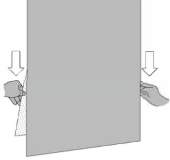
Align the graphic on the surface and use finger pressure to tack it in place.
