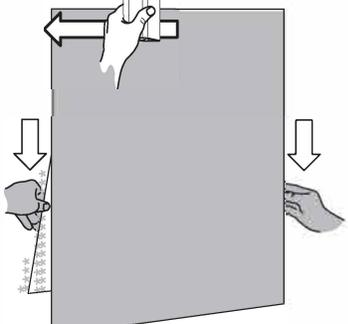
Re-stroke the outer 3 inches of the entire graphic to ensure good edge adhesion.
