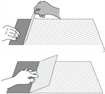
Move the squeegee over a couple of inches and continue stroking center to top, center to bottom, as the helper pulls the liner away from the film.
