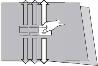
Bring the graphic to the surface and align it along the vertical edge. Use finger pressure to tack it in place. **DO NOT USE TAPE**
