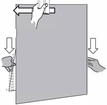
Lay the graphic image side down on a flat surface. Pull back about 6 inches of the liner. Sharply crease the liner.
