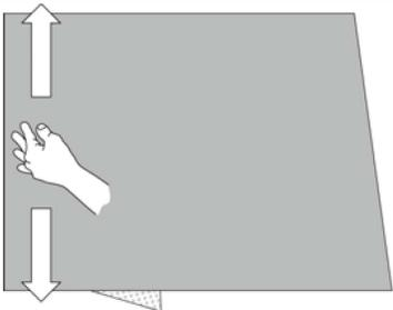
Re-stroke the outer 3 inches of the entire graphic to ensure good edge adhesion.
