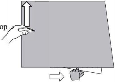
Lay the graphic image side down on a flat surface. Pull back about 6 inches of the liner. Sharply crease the liner.
