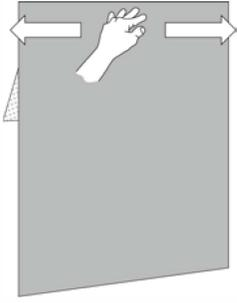
Move the squeegee down a couple of inches and continue stroking right and left, pulling the liner down as needed. Repeat to the bottom.
