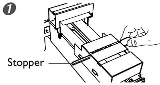
Install the stopper in this groove.
