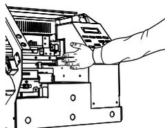
Touch the location shown in the figure to discharge any static electricity.
